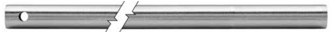
Top Rod - 2200 and FL2200 Series. Three stock lengths available for 7'-0", 8'-0", and 10'-0" high doors. TR1854 – For 7'-0" doors, rod is 36" long. TR1855 – For 8'-0" doors, rod is 48" long. TR1857 – For 10'-0" doors, rod is 72" long. For doors of lesser height rods must be field cut. Specify finish (see page 3 for Finish Descriptions).
